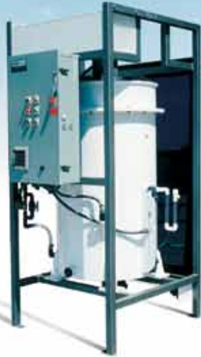
MS MiniScrubber with a simple, sparger tube design; 500-6,000 ACFM. Used for lab hoods, core machines and process tanks.
